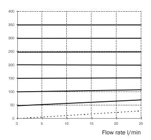
... = min. setting pressure max. setting pressure 350 bar
