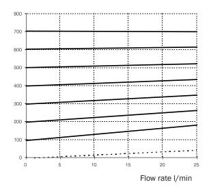
... = min. setting pressure max. setting pressure 700 bar
